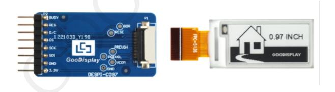
Figure 2: Connection of E-paper display and Adapter
