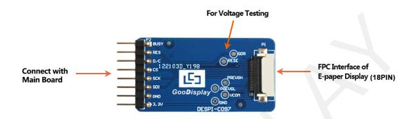
Figure 1 DESPI-C097(18PIN)
